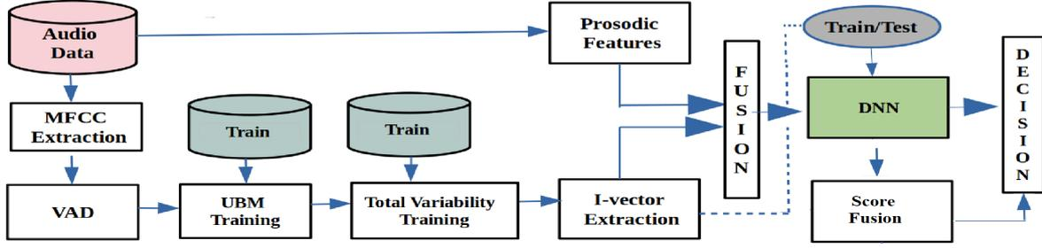
Figure 2: Block diagram of the the proposed system
